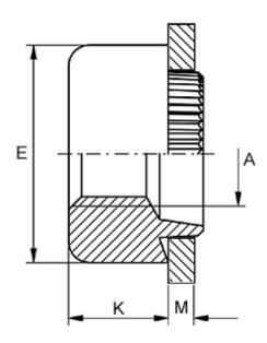
Female thread A = M12 Height K = 10.0 Outer diameter E = 25.0 Plate thickness = 0.9 to 1.0
